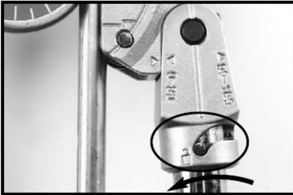
**Рис. 12 - Позиция "Unlock"**
